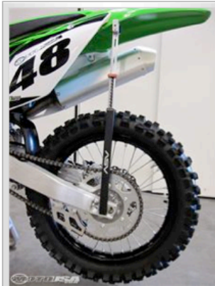
The ASV Solo Sag Scale is the simplest way to measure rear suspension sag
