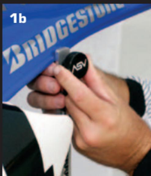
not scratch your fender or graphics. Failing to tighten the clamp as much as possible will result in the Solo Sag Scale slipping off your rear fender.
