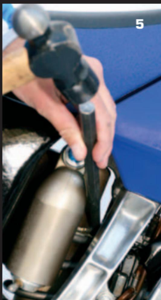
Directly above the spring on your rear shock are two lock rings that tighten up against each other. Both of these lock rings have notches in them to allow you to use a punch (or large flat screwdriver or small tire iron, etc.) to turn them. Using the punch
