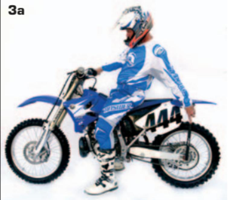
the rear wheel up off the ground and your rear suspension fully extended. Your Solo Sag Scale will now be displaying the rider sag measurement (Photo 4a & 4b).
