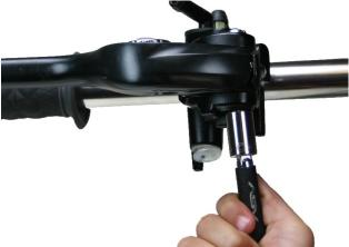
1b) Remove the lever. If the plunger rod comes out, re-insert it back into the master cylinder.
