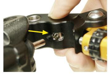
2b) Place the pivot bolt back into the master cylinder and tighten. Secure with the 10mm nut underneath. Do not overtighten.
