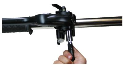
1b) Once removed, unscrew the pivot bolt and remove the lever. If the plunger rod comes out, place it back into the master cylinder.
