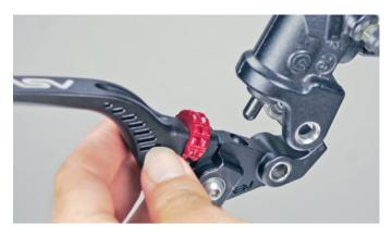
2b) Use the flat head screwdriver to screw in the pivot bolt. Secure with the 10mm nut underneath. Do not overtighten.
