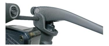
1b) Remove the lever. Be careful as the OEM push rod may also fall out of the master cylinder.
