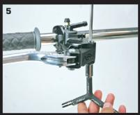
locknut as it can cause binding of the lever and master cylinder. Maximum torque on locknut should be five (5) foot-lbs. or sixty (60) inch-lbs.
