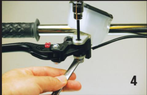
**AFTER INSTALLATION** with the engine off and bike out of gear, apply the front brake several times to confirm it is functioning properly. You should hear the “clicking” sound of the brake light switch being activated each time you pull the brake lever in. There should be no drag and the front wheel should spin freely when brake is not engaged. With the Key in the “ON” position, your rear brake light
