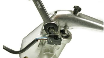
1b) Remove the 4mm hex pivot bolt. The lever and the push rod should removable.
