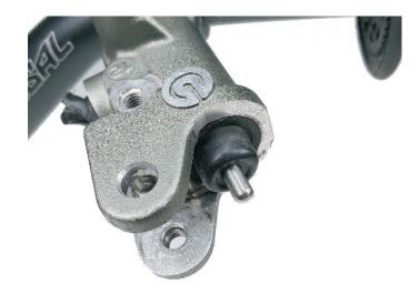
2b) Place the ASV into the master cylinder, making sure that the push rod sits inside the barrel of the ASV lever.
