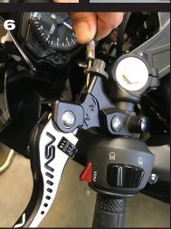
AFTER INSTALLATION is complete, with the engine off and bike out of gear, apply the clutch several times to ensure it is functioning properly. There should be no drag or binding when the clutch lever is pulled. Test your neutral safety switch by placing the key in the "ON" position, placing your bike in neutral, and attempting to start the bike. The bike should only start with the clutch engaged. If something does not seem right, contact ASV technical support before riding your motorcycle.
