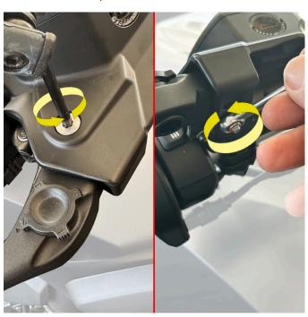
3b) Once the nut is off, use your fingers or a flathead screwdriver to push or pull the Torx bolt out of the master cylinder. Carefully remove the lever from the master cylinder.
