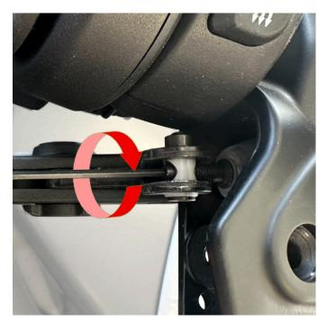
3e) Once released, remove the barrel-shaped retainer.
