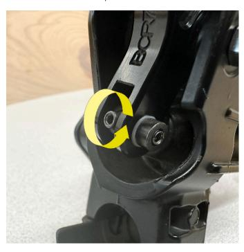
4c] Use the 2mm hex key wrench to tighten the push rod retainer screw until the colored threads are no longer visible or flush.
