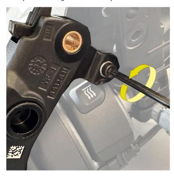
3d) On the inside of the lever, use a 2mm hex key on the push rod screw and turn CLOCKWISE until the lever is released.
