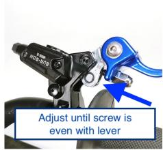
Adjust the screw until it is even with the lever
