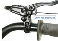
Use the 2mm hex to loosen the reach adjuster screw all the way out.
