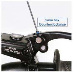
Use a 2mm hex wrench to remove the retainer screw located on top of the lever.
