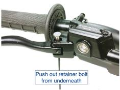
Push out the retainer bolt from underneath
