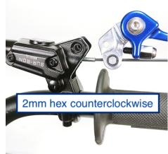
Use a 2mm hex counterclockwise to screw in the ASV lever
