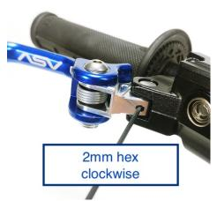
Tighten the retainer screw on the ASV lever
