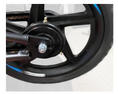
Test the install by spinning the rear wheel. It should spin freely. If struggling, try adjusting at the brake lever before adjusting at the brake cable arm.
