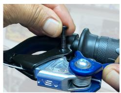
Use the original nut and bolt to secure the ASV lever to the perch.
