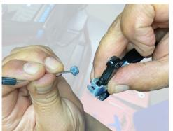
Remove the brake cable barrel from the brake lever.
