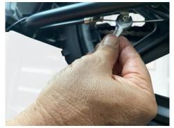
Start at the rear of the bike, underneath the swingarm is a nut that holds the brake cable. Use the 10mm wrench to loosen the brake cable nut.
