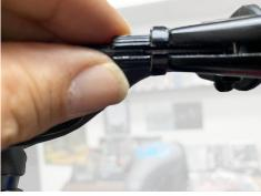
On the handlebar perch, loosen the cable adjuster locknut and tighten the cable adjuster all the way into the perch. Line up the openings to pull the cable out from the perch.
