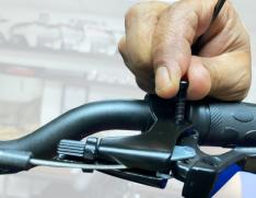
Use a 4mm hex to remove the bolt holding the lever on the perch. Carefully remove the lever, making sure to keep the nut, bolt and spring.
