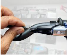
Insert the brake cable back into the perch and tighten the brake cable adjustor all the way.
