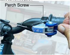
Install the brake cable barrel and the perch spring into the ASV brake lever. Install the ASV brake lever fully into the perch.
