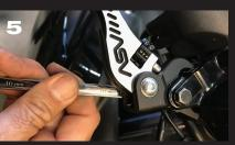
AFTER INSTALLATION is complete, with the engine off and bike out of gear, apply the front brake several times to ensure it is functioning properly. There should be no drag and the front wheel should spin freely when brake is not engaged. With the Key in the "ON" position, your rear brake light should light up when the front brake is applied. If something does not seem right, consult your mechanic or contact ASV technical support before riding your motorcycle.
