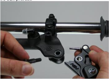
2b) Use a 10mm wrench and flathead to tighten the locknut on the underside of the master cylinder. Do not overtighten.
